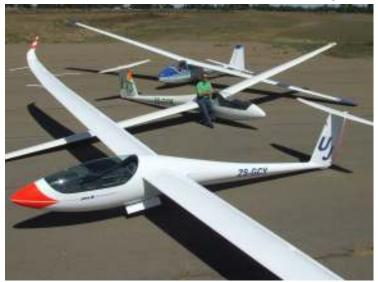
Like dolphins in the water, sailplanes are designed to slice through the air with the absolute minimum of resistance. They represent the leading edge of aircraft design, and the use of modern composite materials, years and even decades ahead of powered aircraft. For example, both winglets and carbon fiber were first used in sailplanes, and only much later adopted in other aircraft.
